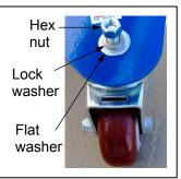
Step 3: Install the remaining caster and strap tab. Install a flat washer before connecting the yellow pull tab, and then install the TAB-BO, if you will use the nylon strap to pull the dolly, or TAB-TH, if you will use an optional rigid hook, followed by another flat washer, a lock washer and a nut. Tighten the nut against the lock washer.
